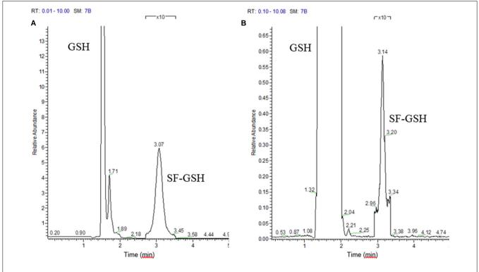
FIGURE 2 | Selected ion monitoring of (A) standard glutathione (GSH) and the sulforaphane-glutathione complex (SF-GSH); (B) Glutathione reaction with microbiota treated with glucoraphanin.
