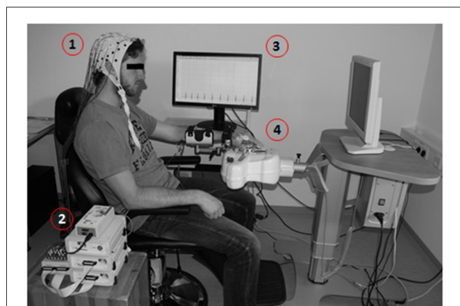
FIGURE 1 | Brain-machine interface (BMI) training environment presented with a healthy subject. Motor imagery (MI)-related modulation of oscillatory activity is detected by electroencephalogram, EEG (1), amplified (2) and processed in a BCI2000-based control system (3) to operate a commercially available electromechanical hand orthosis (4).
