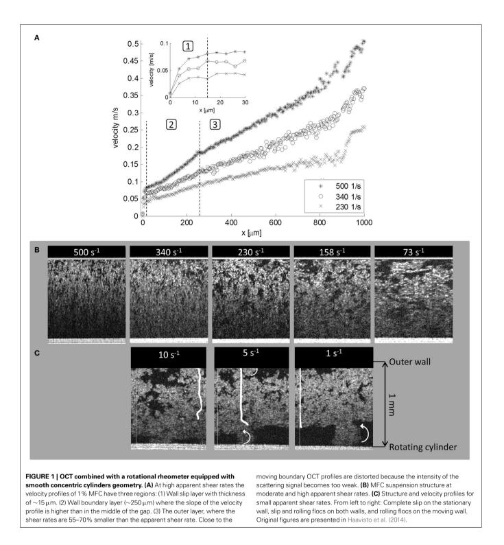
distance of OCT the measurements can be complemented by measuring the outer flow velocity profile with e.g., PUDV or MRI techniques (Salmela et al., 2013). Combining such data with the structural information opens truly unprecedented research prospects for the study of rheology of opaque fluids.
