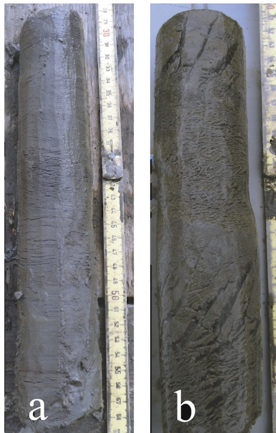
Fig. 12. Examples of cryostratigraphic features in frozen core samples from sites F and A: (a) wavy non-parallel layered cryostructure with fine/thin ice lenses and organic matter layers (F2 depth 1.28–1.58 m); (b) wavy non-parallel layered or lenticular cryostructure (A depth 0.55–0.75 m). Photo scales are in centimeters.
