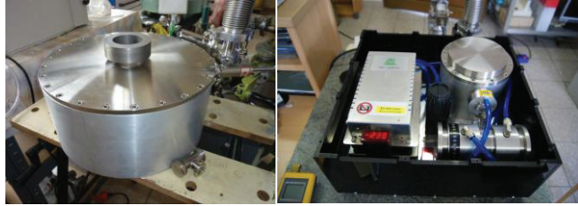
Fig. 1. Mobile HTS magnet platforms with LN 2 and Stirling cryo-cooler (right).
