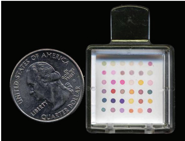
FIGURE 1. Example of colorimetric sensor used in Ref. 31. Chemoresponsive dyes are impregnated on the disposable cartridge. The dye colors change based on the chemicals that adhere to them.
