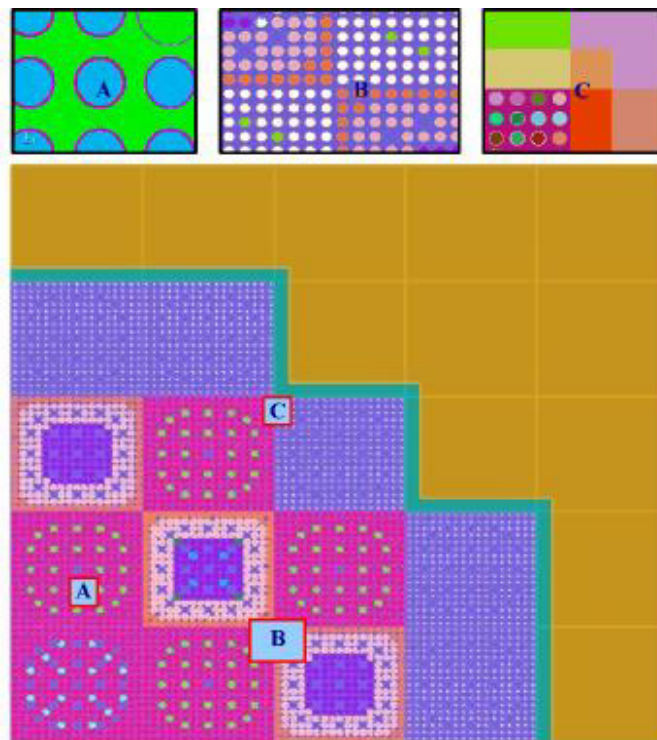
Fig. 8. Benchmark geometry of 1/4 pressurized water reactor with closeup views A, B and C showing details of the model.
