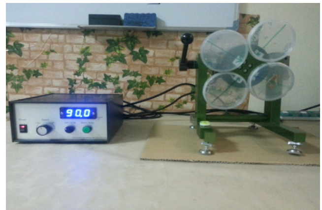
Fig. 1 – Experimental setup of one-axis clinostat.
