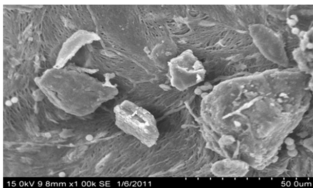
Figure 7 Scanning electron microscope (SEM) image of Metapenaeus monoceros shell biomass.
