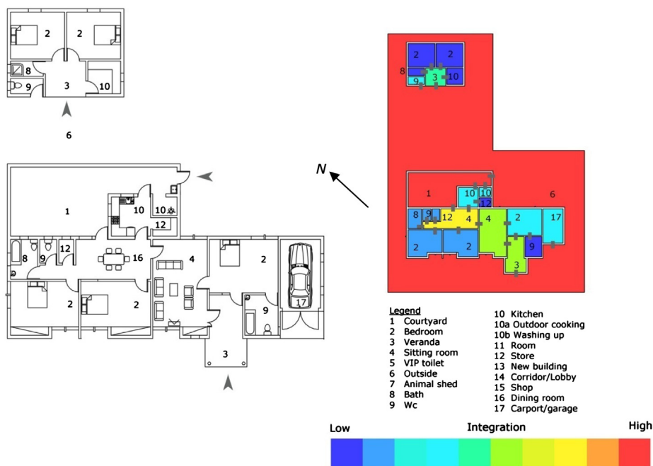
Fig. 14 Pro II floor plans (1:250) and convex map (1:400).
