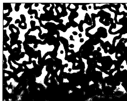
Figure 5. EBIC micrograph showing antiphase boundaries in a GaAs/Ge solar cell. Courtesy Professor D B Holt, Imperial College, London
