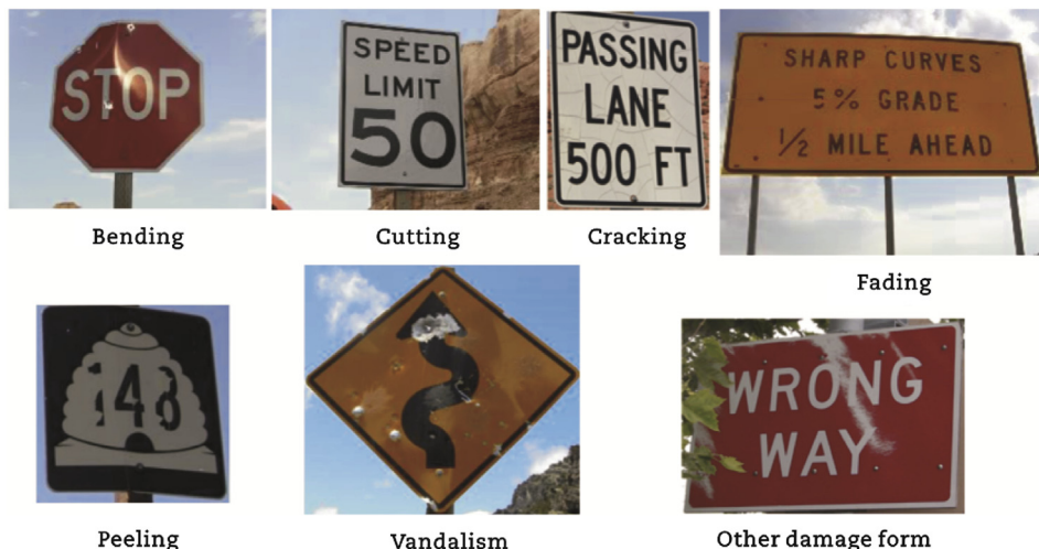
Fig. 4 – Traffic sign damage categories.
