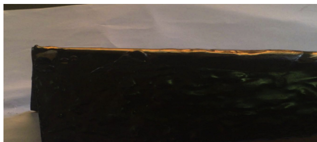
(b) Oxidized asphalt (OA).
