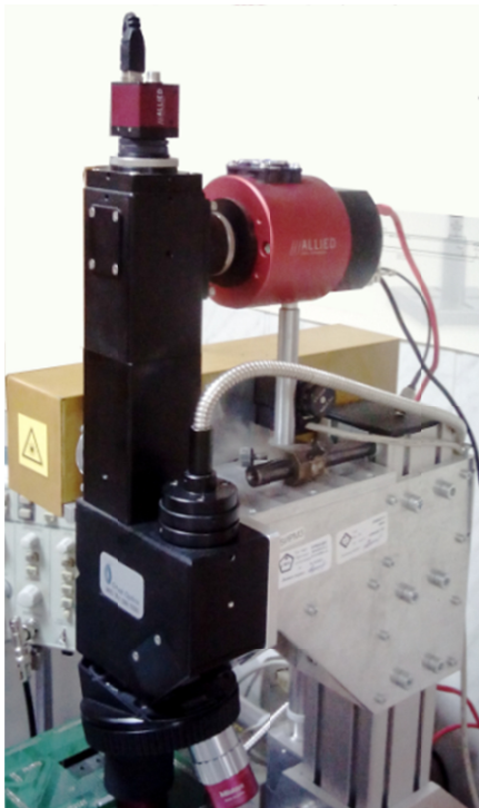
Fig. 2. Microscope with two video-channels (general view).
