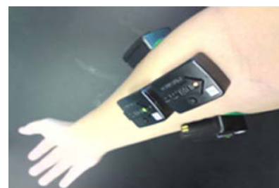
Fig. 3. Placement of the electrode on the subject's forearm
