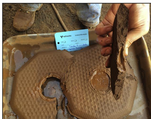
Fig. 7 – Images of actual cake obtained from the laboratory filter. The best cake moisture was obtained for a cake thickness of 35 mm.
