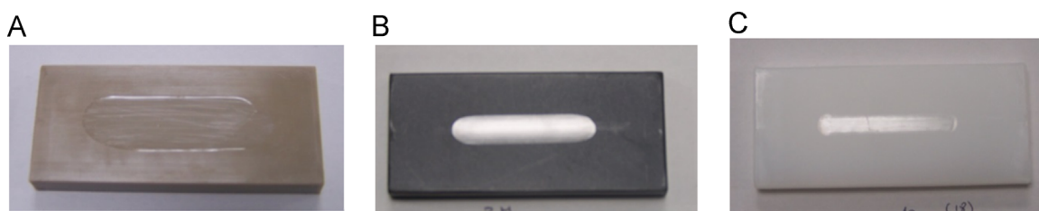
Fig. 5 – Comparison of wear scars on polymer plates after 1Mc (A: PEEK, B: CFR-PEEK, C: UHMWPE).
