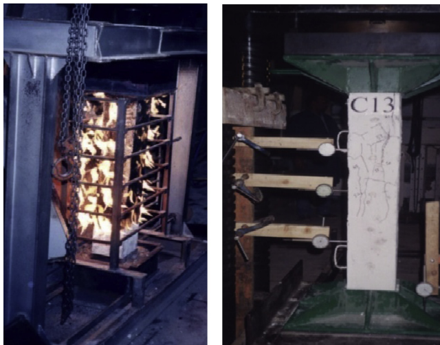
Figure 1 Loading frame, firing cage and column during test.
