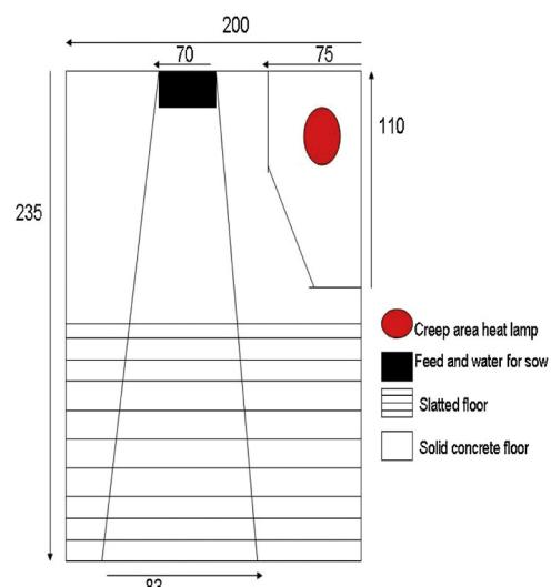
**Fig. 2.** The farrowing crate (all measures in cm).
