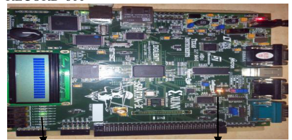
Fig14:Green Light(LED-E9) indicating the detected one as NORMAL SINUS RHYTHM
