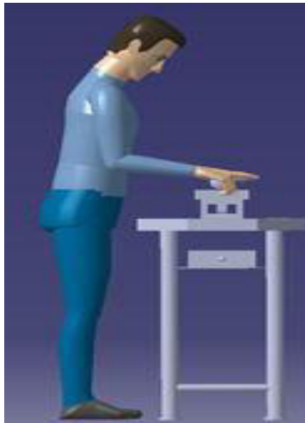
Fig. 3. Mold Scraping Using Proposed Workbench
