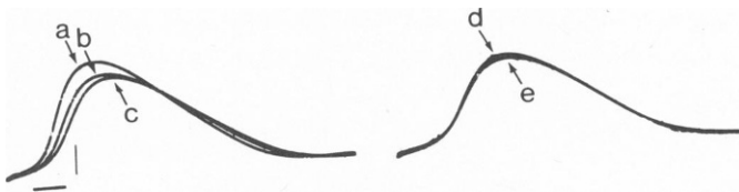
FIGURE A-1 The effects of univalent cations used as \text{Na}^+ substitutes on the monophasic compound action potential of the desheathed frog sciatic nerve trunk. All test solutions contained 1.8 mM \text{Ca}^{2+} and 3 mM \text{Mg}^{2+} and were buffered to pH 6.5–6.6 Stimuli were delivered to the proximal end of the nerve trunk across a petroleum jelly seal separating two pools of full \text{Na}^+ Ringer's solution. Stimulus intensity was adjusted to recruit only the largest diameter ( A\alpha ) fibers. The action potential was recorded across a seal separating a pool containing the test solution and a pool containing full (116 mM) TMA Ringer's solution. ( a ) Full \text{Na}^+ Ringer's solution; ( b ) 51 mM TMA Ringer's solution; ( c , d ) 51 mM glucosamine Ringer's solution; and ( e ) 51 mM arginine Ringer's solution. Calibration 0.1 ms \times 5 mV.
