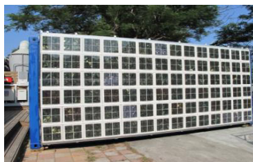
Fig. 3 The 1kWp BIPV system was hang on the front surface of a container of transportation
