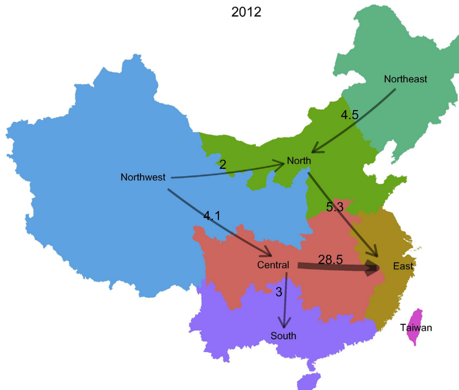
Fig. 1. The inter-regional transmission grid in 2012. Note that the numbers close to the lines indicate transmission capacity (in GW), and the arrows reflect the main directions of power flows. The data are compiled by the authors with data in [3,8].
