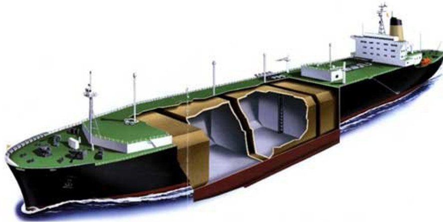
Fig. 1 Membrane-type LNG carrier with insulation system.
