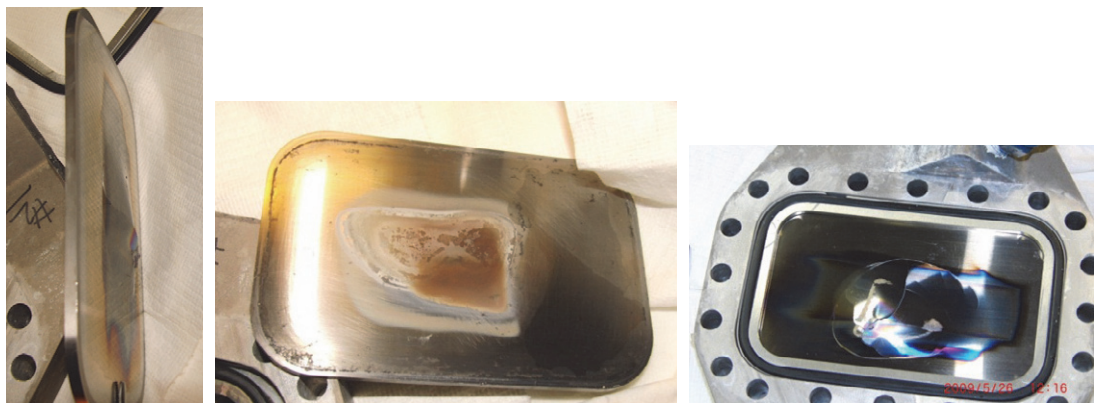
Fig. 6. Hydrogen impregnation failure at 13 MeV
