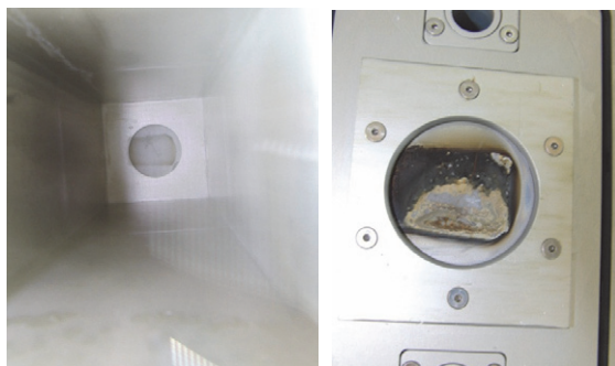
Fig. 14. New Target failure; beam side on left and water side on right.
