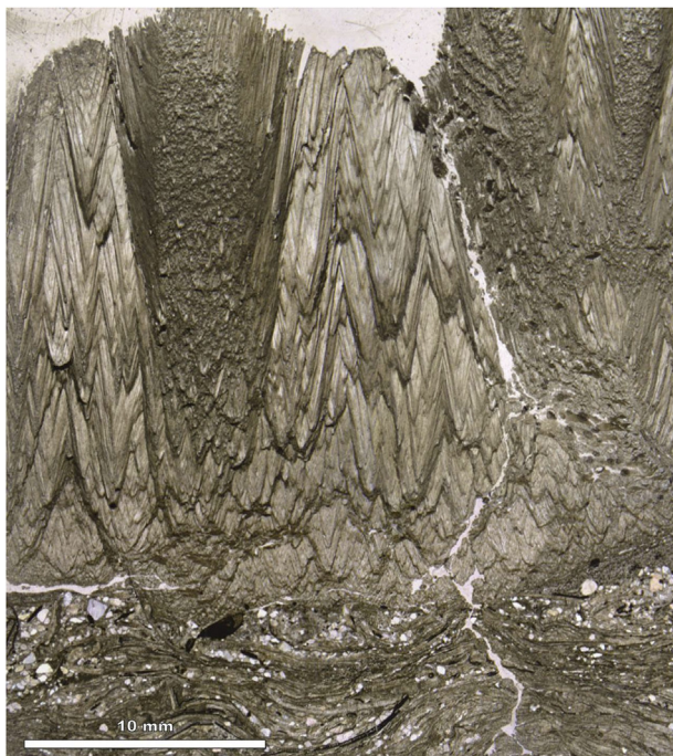
Fig. 6 – Vertical thin section view of upper limestone bed at Lavernock Point showing upward growth of CIC calcite crystals from the shelly limestone bed. The sharp contact between the shelly limestone and the CIC calcite may be evidence of growth of the CIC calcite layer as additive, in a fracture. On the upper right side of the photo, the upward-protruding crystal mass is part of a “nailhead” in vertical section (see also Fig. 3C).
