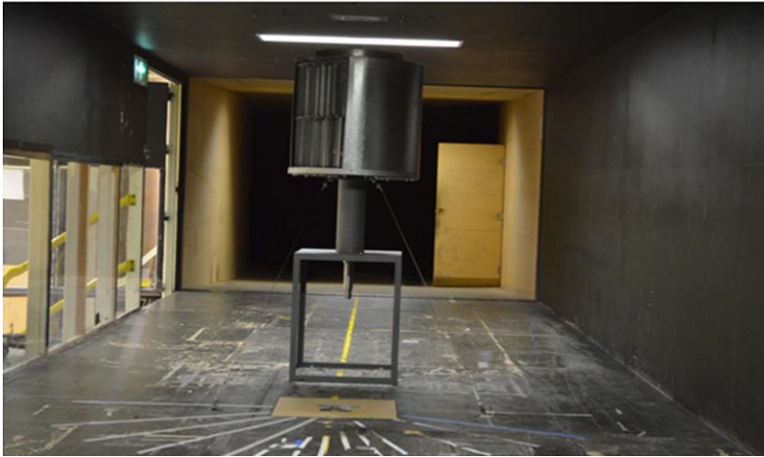
Fig.3. Wind turbine prototype made from stainless steel.
