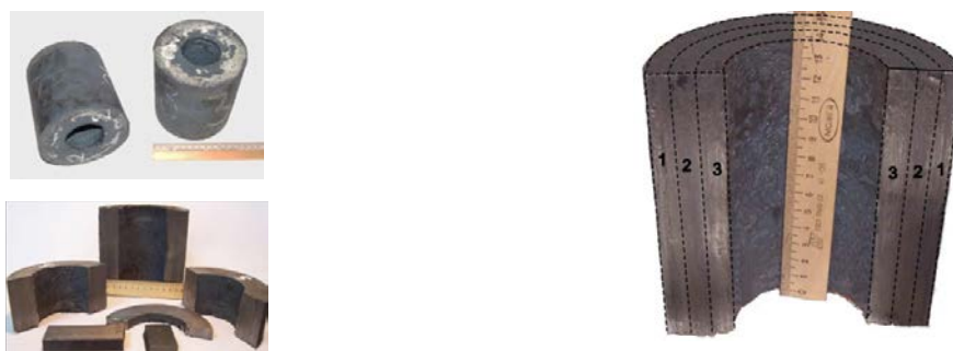
Fig. 1. Fabricated cylinders and cut-out samples: 1 – outer zone, 2- ½ of the width, 3 – inner zone.
