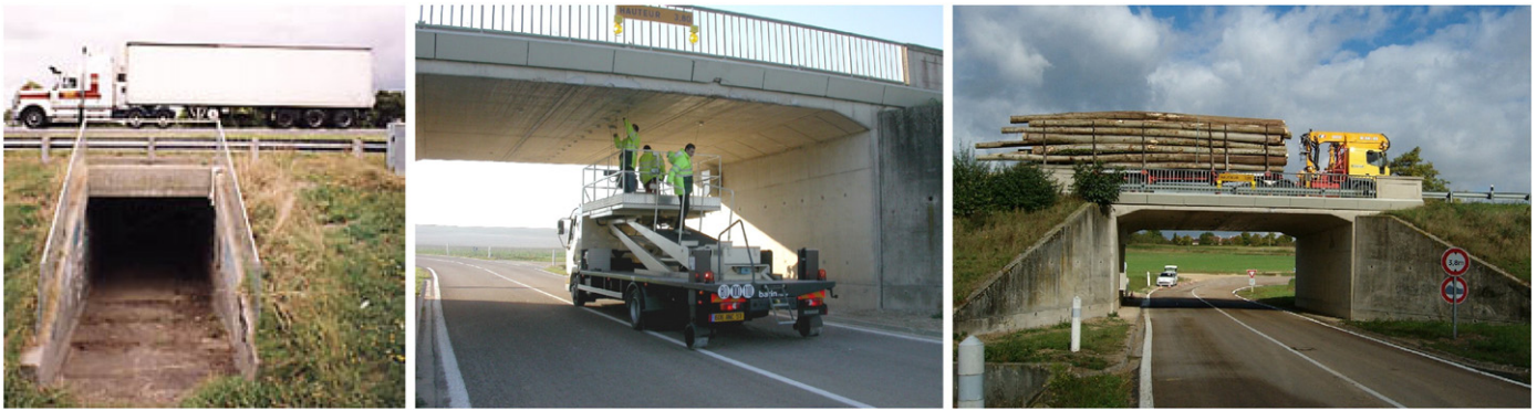
Fig. 8. B-WIM: culway in Australia (left), instrumentation (center) and measurement (right) on an integral bridge in Nogent-sur-Seine, France.
