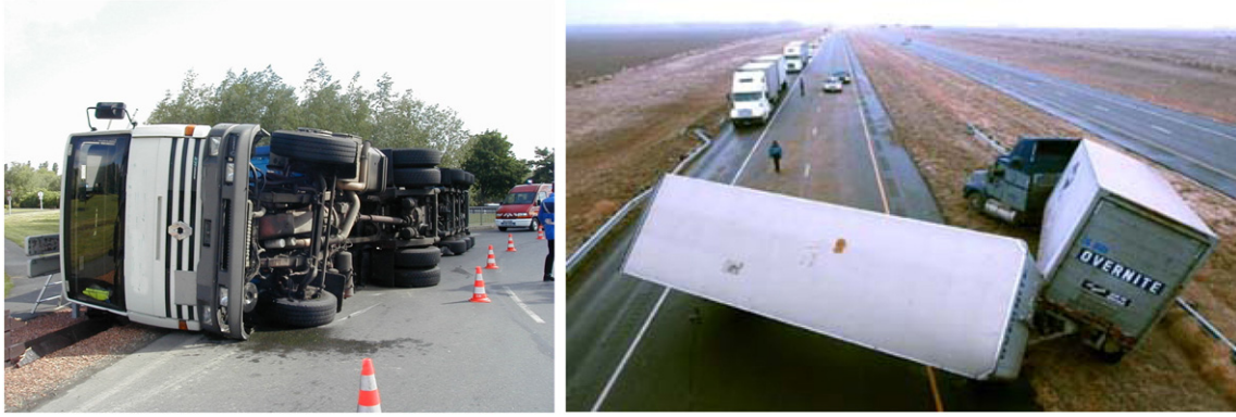
Fig. 1. Truck rollover and knife-jacking.
