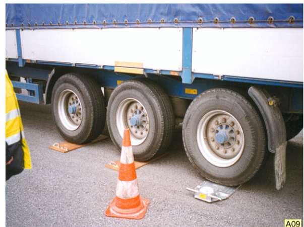
Fig. 3. Portable static wheel scales and leveling wood plates.
