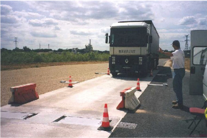
Fig. 4. Low Speed WIM using load cell wheel scales in a concrete platform (Châlons / Saône, France).
