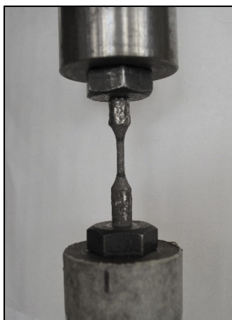
Fig. 2. Static tensile test.
