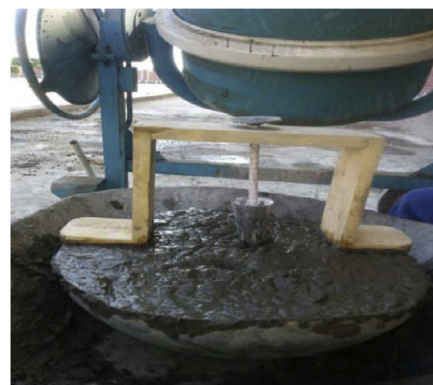
b- Cone penetration test in progress
