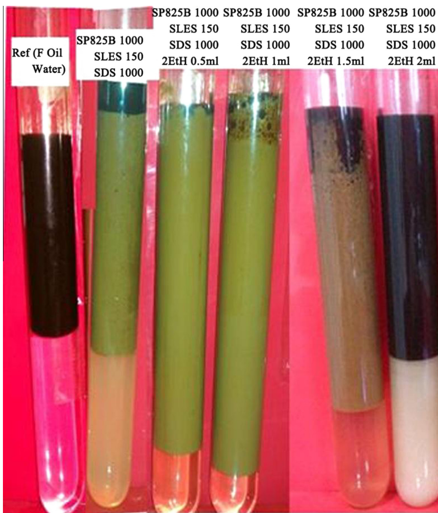
Figure 7 The phase behavior of water and F oil in the presence of SP825B polymer, the combination of SLES/SDS surfactants and 2-ethylhexanol alcohol after 24 h exposure to the heat treatment (90 °C) (the written numbers represent surfactant concentration (ppm) within the total volume of water and oil).
