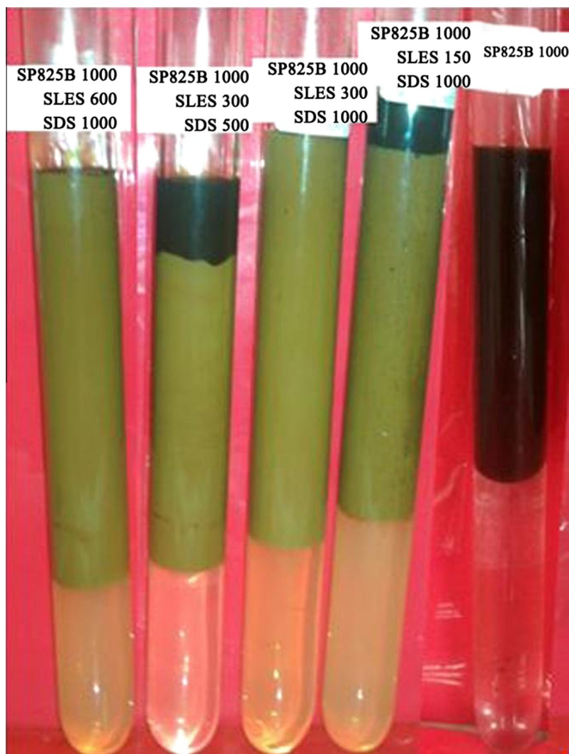
Figure 6 The phase behavior of water and F oil in the presence of SP825B polymer and the combination of SLES/SDS surfactants after 24 h exposure to the heat treatment (90 °C) (the written numbers represent surfactant concentration (ppm) within the total volume of water and oil).
