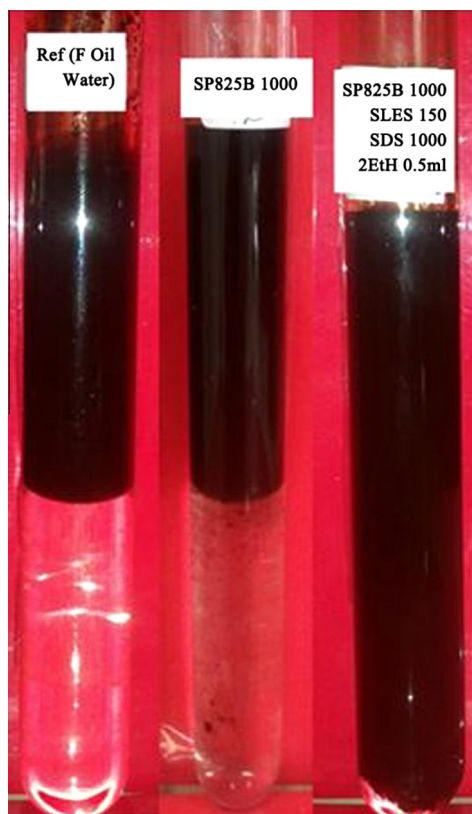
Figure 10 The phase behavior of water and S oil in the presence and absence of polymer, the combination of SLES/SDS surfactants and 2-ethylhexanol alcohol after 24 h exposure to the heat treatment (90 °C) (the written numbers represent surfactant concentration (ppm) within the total volume of water and oil).
