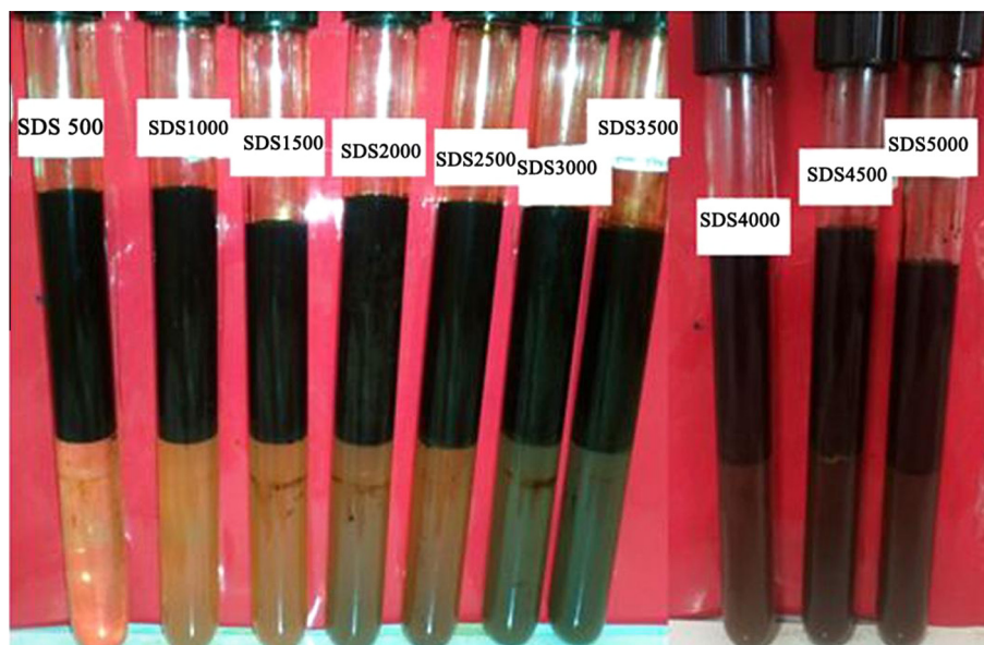
Figure 5 Phase behavior of water and S oil in the presence of SDS surfactant after 24 h exposure to the heat treatment (90 °C) (the written numbers represent surfactant concentration (ppm) within the total volume of water and oil).
