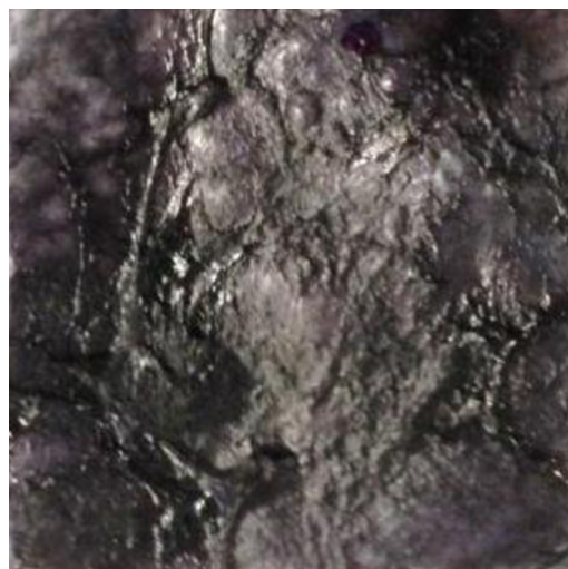
Fig. 1. PEC film obtained from chitosan and pectin suspensions containing a colourimetric bioactive compound (ATH).
