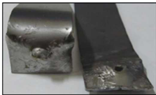
Fig. 11. Nugget Pull in specimen PSet06
