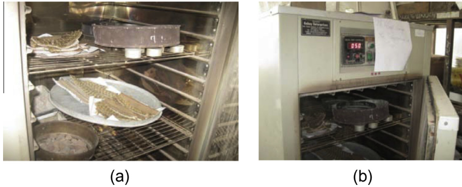
Figure 1. (a) Samples in oven for high temperature conditioning; (b) thermostatically controlled oven used for heat treatment of woven natural fabrics.
