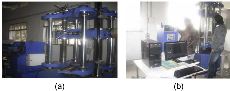
Figure 6. (a) Instrument used for compressive testing of cylinders; (b) the instrument along with the digital data acquisition system.
