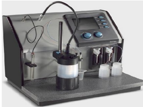
Fig. 2. Zeta potential instrument of thick grout.
