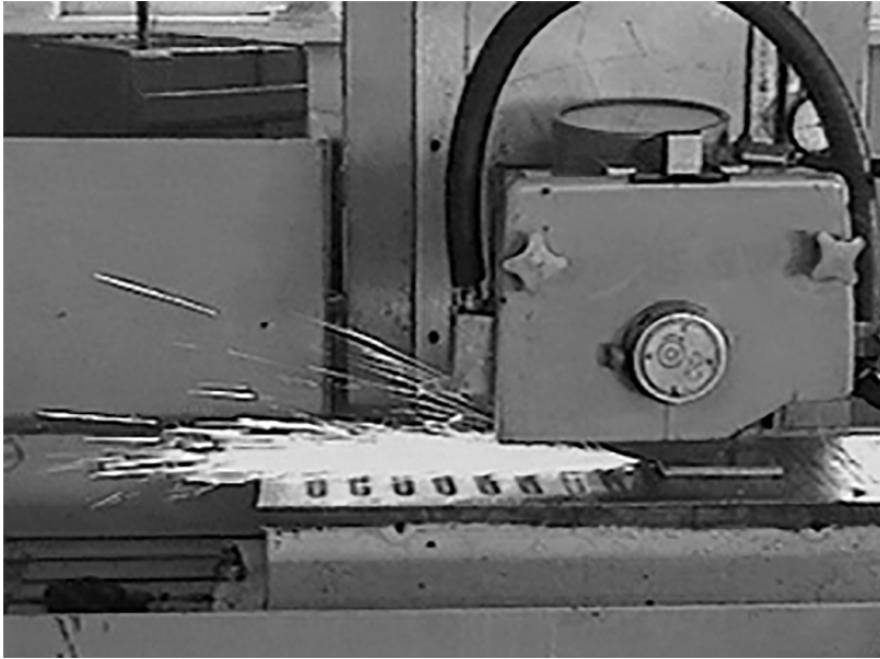
Fig. 6. Directional flow of slurry (Torch), formed by flat grinding
