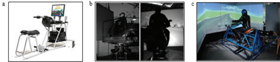
Fig. 4. Examples of established motorcycle simulators: (a) Honda SMARTrainerMotorcycle Simulator [9]; (b) MORIS Motorcycle Simulator [10]; (c) University of Padova Motorcycle Simulator (UNIPD) [11].
