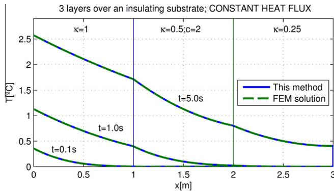
**Fig. 8.** Simulation of a constant heat flux into a three layer material placed over an insulating substrate. In the simulation, all parameter properties of the layers and substrate are the same as in Fig. 5 except their thermal conductivities whose values can be seen in the plot and the specific heat of layer 2 which was set to 2 J/kg. The simulation time can be seen in the graph. Properties in the plot are in SI units.
