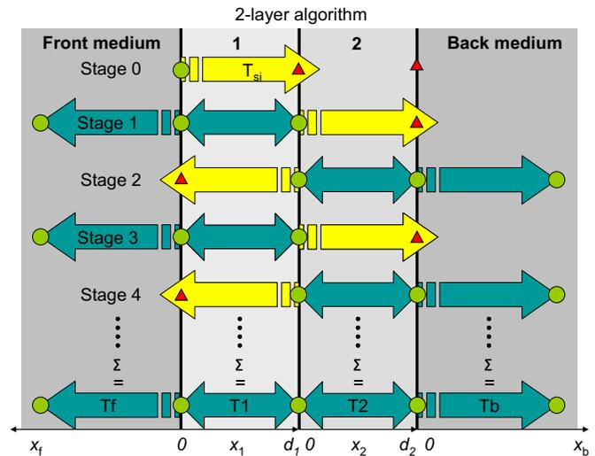
Fig. 5. The 2-layer algorithm based on the successive application of the 1-layer algorithm. For an explanation of the arrows see legend of Fig. 4. The final solutions for each region are the result of the summation of temperature functions represented by dark blue arrows.
