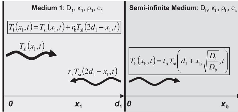
**Fig. 1.** The temperature in two different media assuming a temperature source located in  $x_1 = 0$  of medium 1. The interface between the media is located in  $x_1 = d$  ( $x_b = 0$ ). Parameters  $r_b$  and  $t_b$  can be thought of as the “reflection” and “transmission” coefficients respectively of the temperature solution “incident” on the interface between the media.
