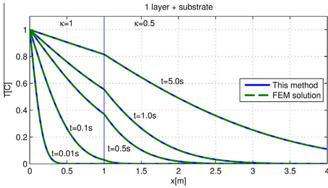
**Fig. 3.** Results of the simulation of a thermal reservoir in contact with a layer over a substrate (Eqs. (27) and (28)). All the parameters for the slab were taken as unity namely: thermal diffusivity  $\kappa_1 = 1$  W/m-K, mass density  $\rho_1 = 1$  kg/m<sup>3</sup>, specific heat  $c = 1$  J/kg-K and thickness  $d_1 = 1$  m. Parameters for the substrate were the same as the layer except its thermal conductivity which is half that of the layer.
