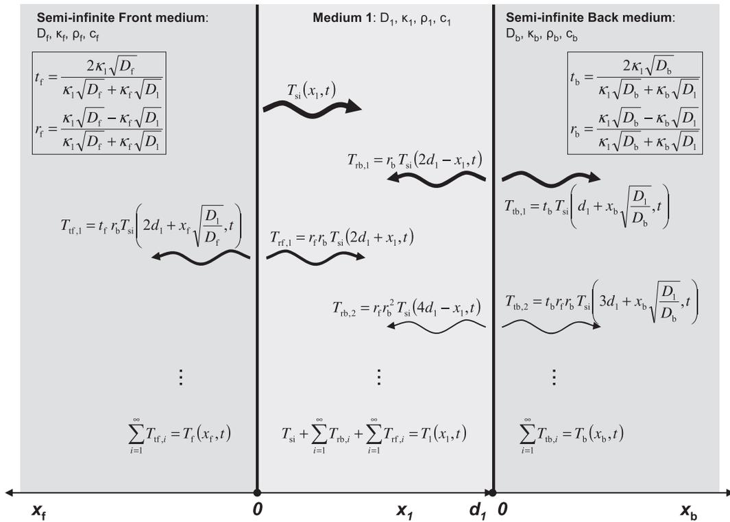
**Fig. 2.** A computation scheme for calculating the temperature for a sandwich structure consisting of a front semi-infinite medium, a layer medium and a backside semi-infinite medium. All media have different thermal properties. We assume a heat source at  $x_1 = 0$  whose temperature function is  $T_{si}(x, t)$  applicable inside the layer medium, considered semi-infinite. This temperature function is assumed to be consistent with the boundary condition at the front face.
