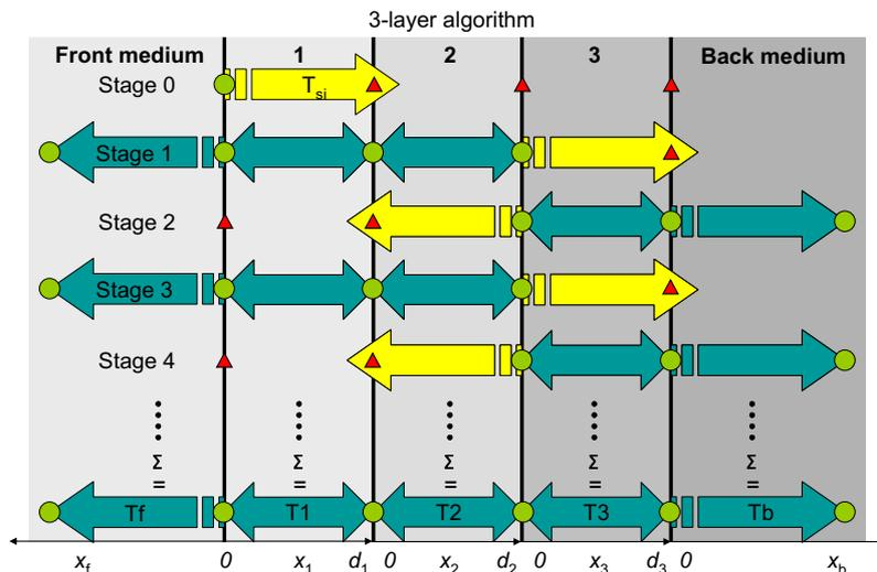
**Fig. 7.** The 3-layer algorithm based on the successive application of the 2-layer and the 1-layer algorithms. For an explanation of the arrows see caption of Fig. 4.
