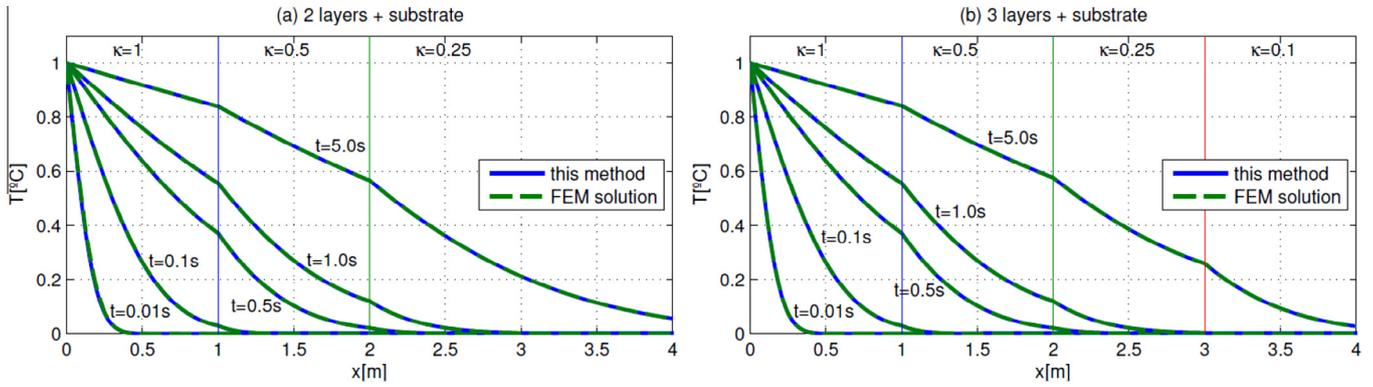
**Fig. 6.** Simulation of an heat reservoir in contact with (a) a two layer over a substrate; (b) a three layer over a substrate. In the simulation, all properties of the layers and the substrate are the same as in Fig. 3, except the thermal conductivity of the layers and the substrate which is indicated in the plot in SI units (i.e. W/m-K). The thickness of the layers is the same and equal to 1 m. The simulation times can be seen in the graphs.
