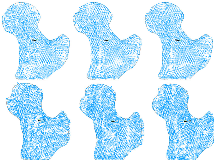
Fig. 9. Maximum principal stress vector plots for micro-FE (left), orthotropic (middle) and isotropic (right) models for the healthy femur (top) and osteoporotic one (bottom).
