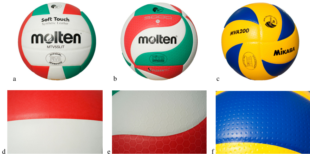
Figure 2. Ball panels (a, b, c) and shape of surfaces (d, e, f) on three type volleyballs for this experiment (a: molten MTV5SLIT, b: molten V5M5000, c: mikasa MVA200).
