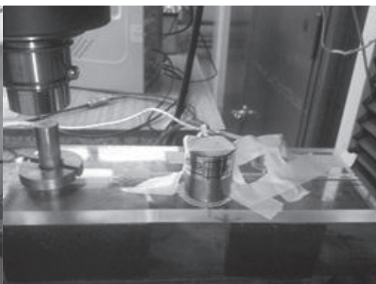
Fig. 2. Experimental set-up: specimen, tensile tool and sensors.
