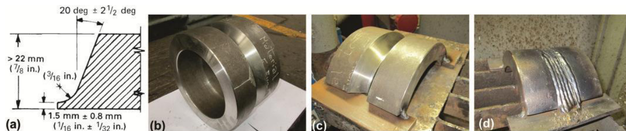
Fig. 1. (a) Geometry of the joint according to ASME B31.3; (b) Pipe machined according to (a); (c) Joint pieces cut at 120 ° and ready to be welded; (d) welded joint.
