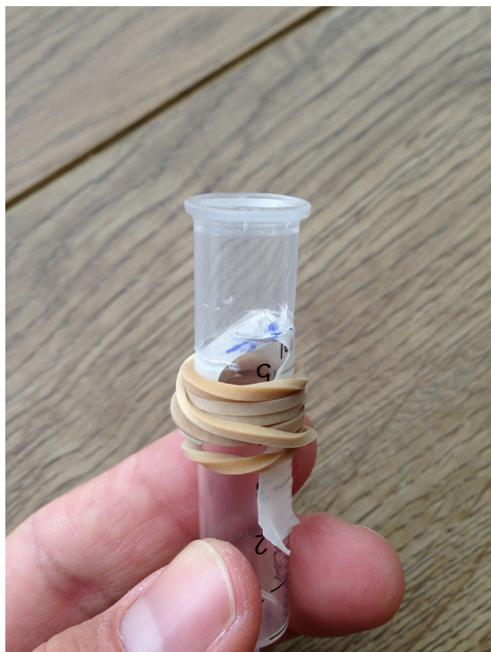
Fig. 2. Latex membrane with an angle of approximately 45° at 25–30 mm depth, to simulate the characteristics of the tympanic membrane.
