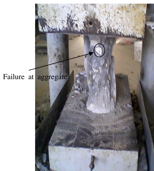
Figure 11 The mode of failure in aggregate.
