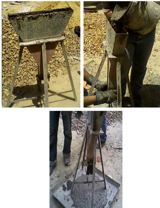
Figure 3 The V-funnel test.
