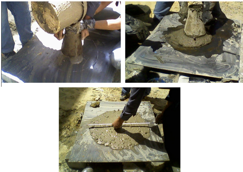
Figure 2 The slump-flow test.
