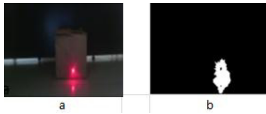
Fig 5: (a) Input image sent to system (b) Segmented Image for laser light detection
