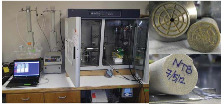
Figure 1. High pressure test system with Hassler sleeve core holder houses 2.54 cm (1 inch) diameter samples up to 15.24 cm (6 inches) long at pressures to 136 bar (2000 psi) (left). After MICP treatment, significant precipitation was observed on the core inlet (not shown) and outlet (right top) as compared to an unmineralized core (right bottom).
