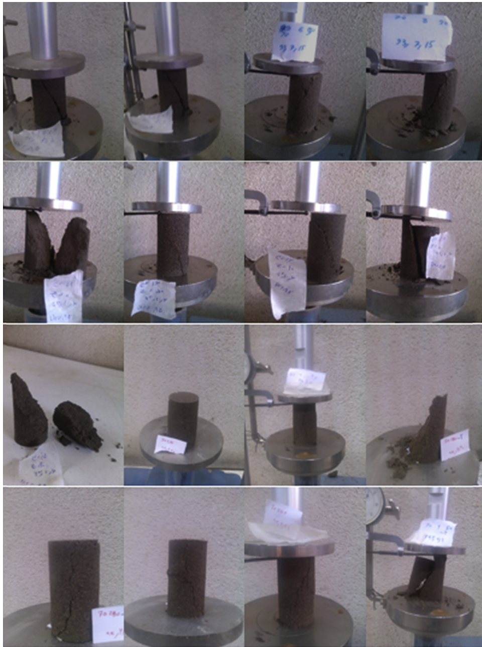
Fig. 2. Failure types of stabilized specimens.
