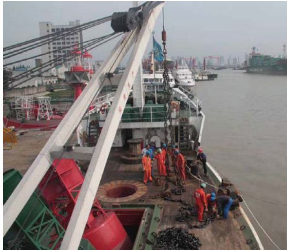
Fig. 1 A special vessel for the buoy deployment
